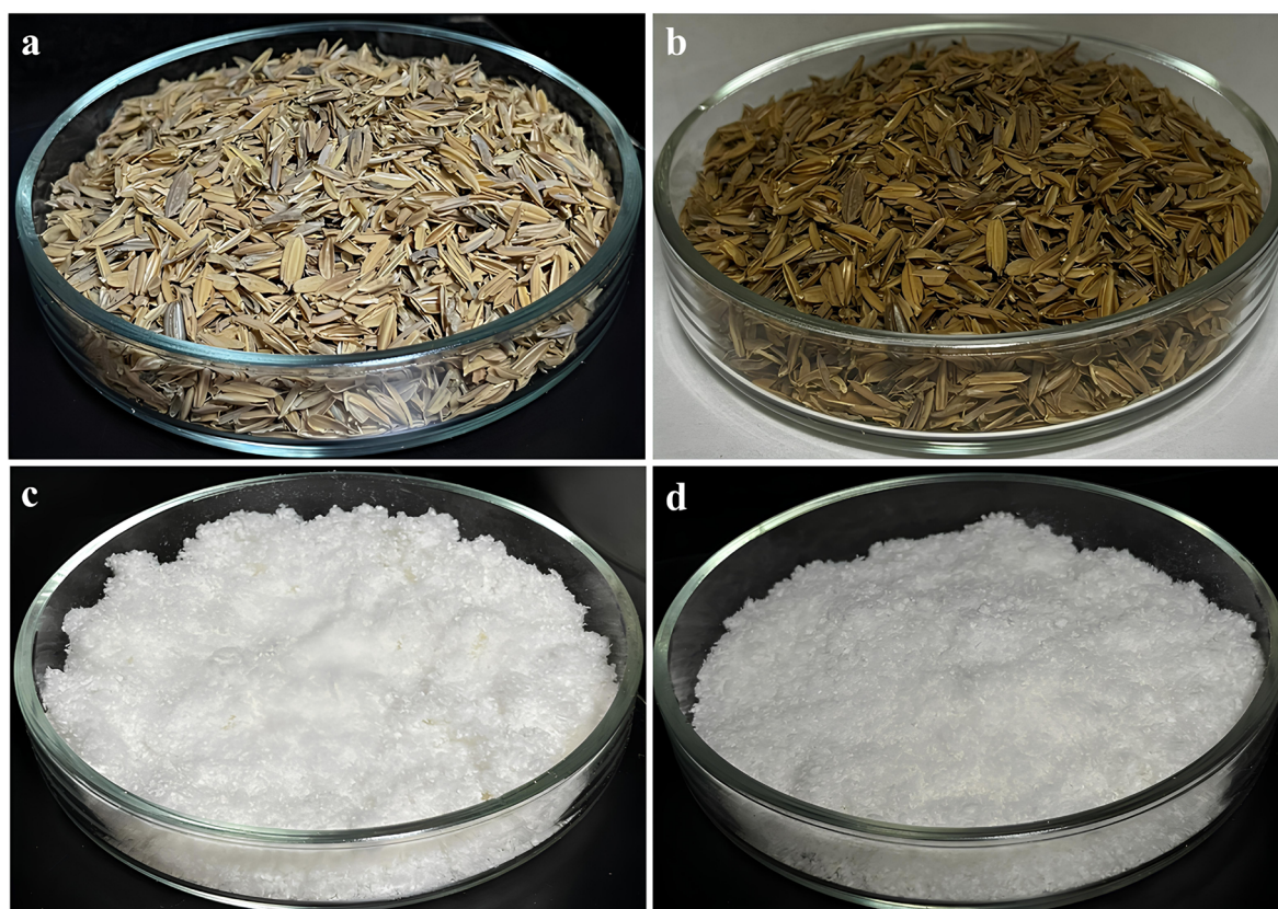
Figure 2 – Rice husks and MCC samples from RH: a – B-RH; b – K-RH; c – MCC B-RH (hydromodule 1:12); d – MCC K-RH (hydromodule 1:10)
